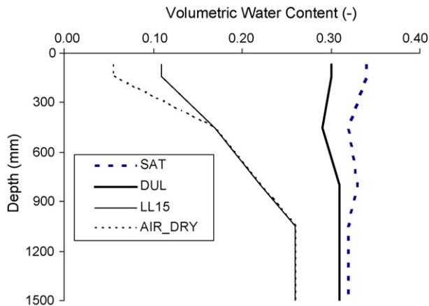
Fig. 1. Soil hydraulic properties of the study site in Simmons Creek, NSW, Australia. SAT, DUL, LL15 and AIR\_DRY are the soil water content at saturation, drained upper limit, lower limit ( $-1500$  kPa matric potential), and air dry water content, respectively (all laboratory-determined).
