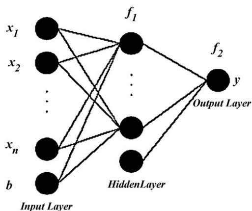
Fig. 3. Topology of a three-layer feed-forward neural network. Redrawn after Lek et al. (1996).
