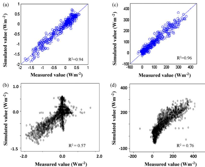
**Fig. 4.** Comparison of the ANN approximations with stepwise linear regressions for CO<sub>2</sub> and water vapor fluxes. (a) ANN approximations for CO<sub>2</sub> flux; (b) stepwise linear regressions for CO<sub>2</sub> flux; (c) ANN approximations for water vapor flux; (d) stepwise linear regressions for water vapor flux.
