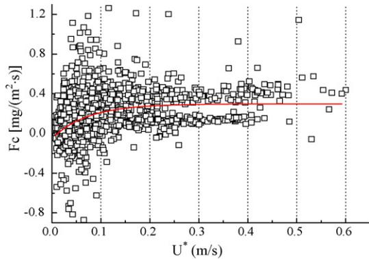
Fig. 1. Measured nighttime  $\text{CO}_2$  flux ( $F_c$ ) vs. nighttime turbulence ( $U^*$ ).
